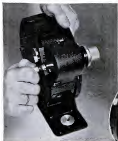
Loading bulk film for miniature-camera use. Right, note footage indicator
